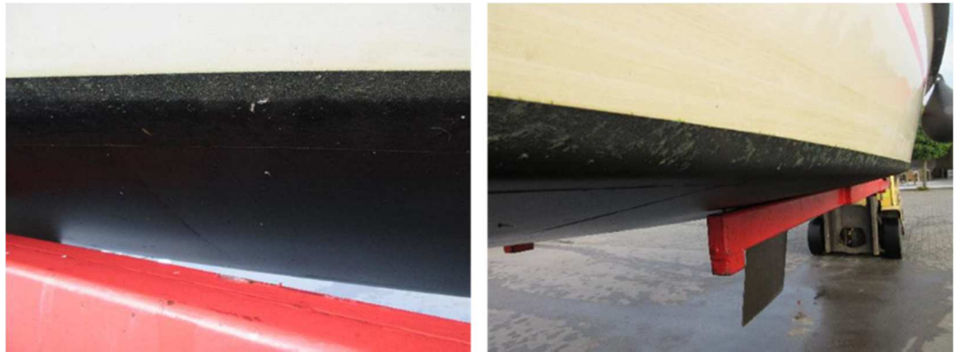
Figure 26. Boat with Finsulate product at the final inspection.
