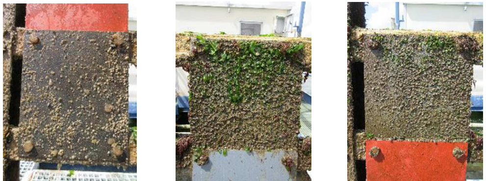
Figure 9. Detailed pictures of panels with Seajet ex3, GPN and blank PVC (from left to right).
