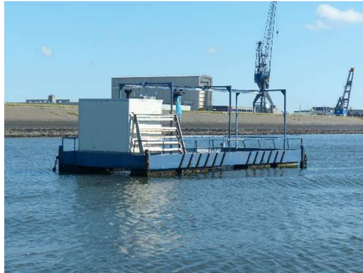
Figure 1. Raft exposure facility of Endures in the harbour of Den Helder, The Netherlands
