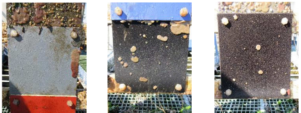
Figure 12. Detailed pictures of panels with Melkfett, Finsulate short and Finsulate long (from left to right).
