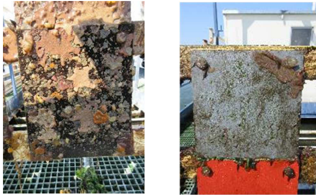
Figure 15. Detailed pictures of panels with Finsulate long (left) and Melkfett (right).
