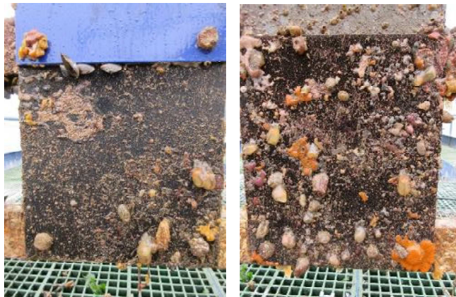
Figure 18. Detailed pictures of panels with Finsulate short (left) and Finsulate long (right).
