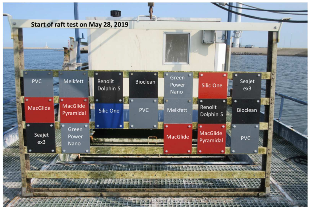
Figure 2. Panels with antifouling products prior to immersion at the raft of Endures.
